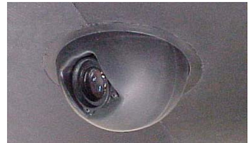
BTC-88R gimbal: (360 degree, 220 grams) 4.5" x 3.5" x 3.5" 10x optical zoom, 4x digital zoom Retractable Diameter: 3.5"
