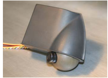
BTC-40 gimbal: (360 degree, 76 grams) 2.75" high (including ball) x 1.5" Wide x 3.5" Long
