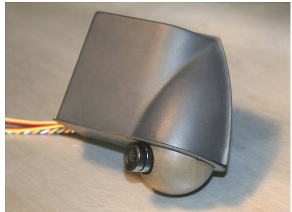
Procerus partner, Brandebury Tool, is the maker of the small gimbal shown above. (360 degree, 76 grams) 2.75" high (including ball) x 1.5" Wide x 3.5" Long
