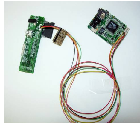
Gumstix processor connected to the Kestrel.
